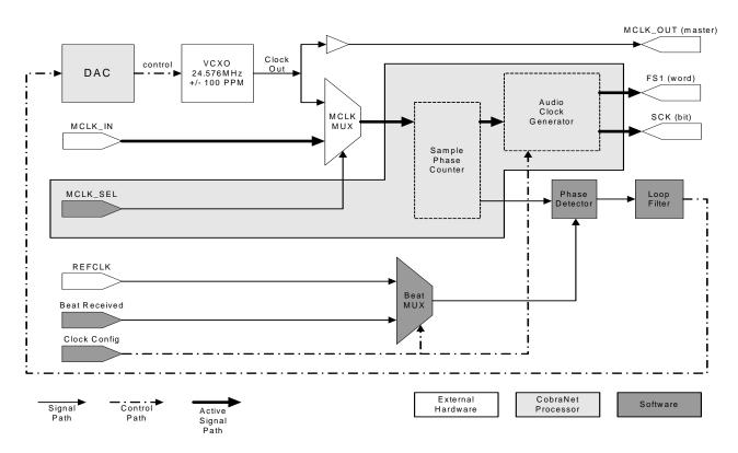
Figure 14. Clock Circuit as Used by Mode 0x04 with CM-2 and Semiconductors
