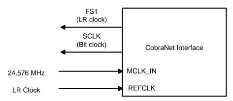
Figure 15. 0x14 Mode Typical Connection (Synchronization to an Externally-Supplied Master Clock and Word Clock when Using CM-1)
