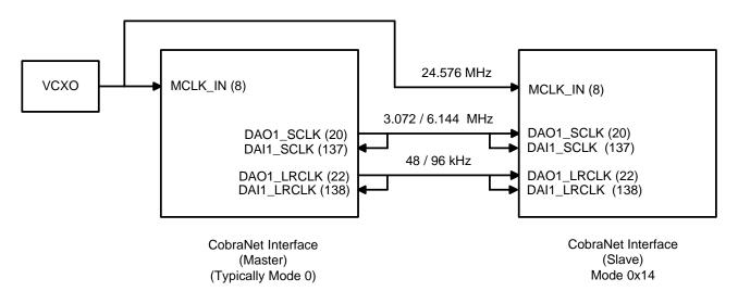
Figure 18. Clock Circuit as Used by Mode 0x14 with CM-2 or Chips with 2x2 or 8x8 Audio Channels
