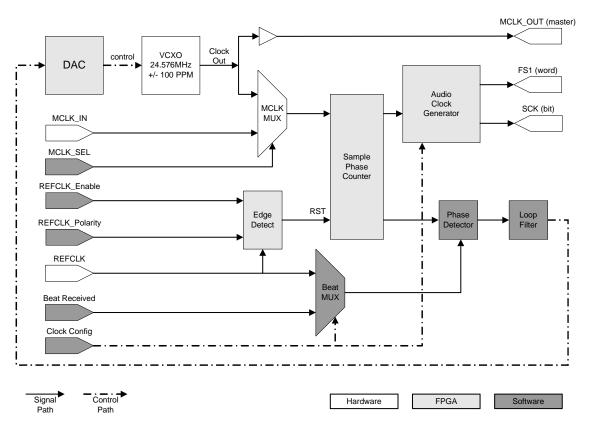
Figure 1. - CobraNet Clock Circuit for CM-1 Module
