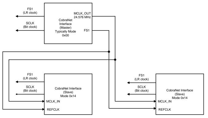
Figure 16. 0x14 Mode Typical Connection
