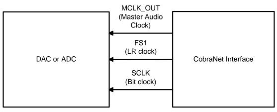
Figure 3. 0x00 Mode Typical Connections
